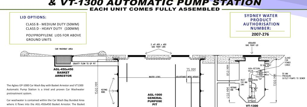
Arrestor removes large matter from the waste stream, protecting the equipment and environment downstream.
